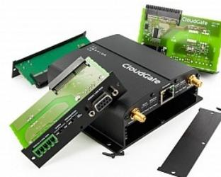
On top of the basic functionality, CloudGate can be tailored to meet specific industrial requirements by adding additional software and peripheral boards. CG9104-900MT is one such peripheral board for CloudGate.
